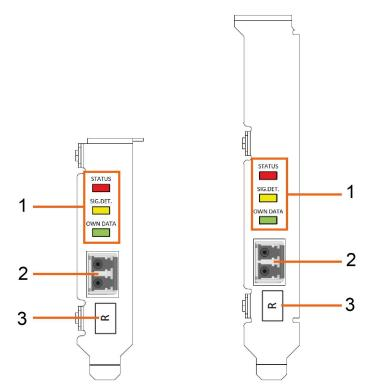
Left: *ibaFOB-R* board with low profile bracket, right: *ibaFOB-R* board with standard bracket
